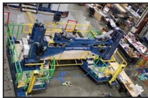
Figure 6. Forward cradle— 1) floating pads allow for roll; 2) cradle driven linearly in X, Y, and Z
