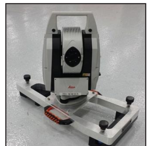
Figure 14. Leica tracker on a custom seat track mount
