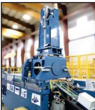
Figure 4. This aft positioner uses a design common to all, providing sub .001-in. repeatability via absolute encoders
